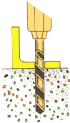
1. Drill hole in concrete (hole dia. same as thread dia.)= (3/8") maximum depth of hole could be any depth beyond minimum recommended depth. Clean out hole of all debris.
